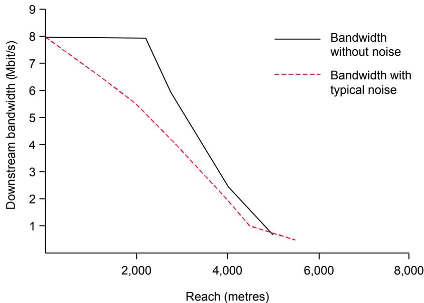
Note: these figures are for 0.5mm copper wiring. Reach depends on the size, age and quality of the wiring used
